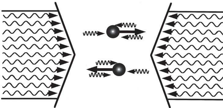
FIG. 12. Doppler cooling in one dimension.
