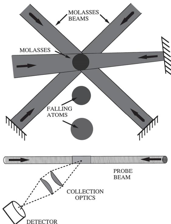
FIG. 15. Time-of-flight method for measuring laser cooling temperatures.
