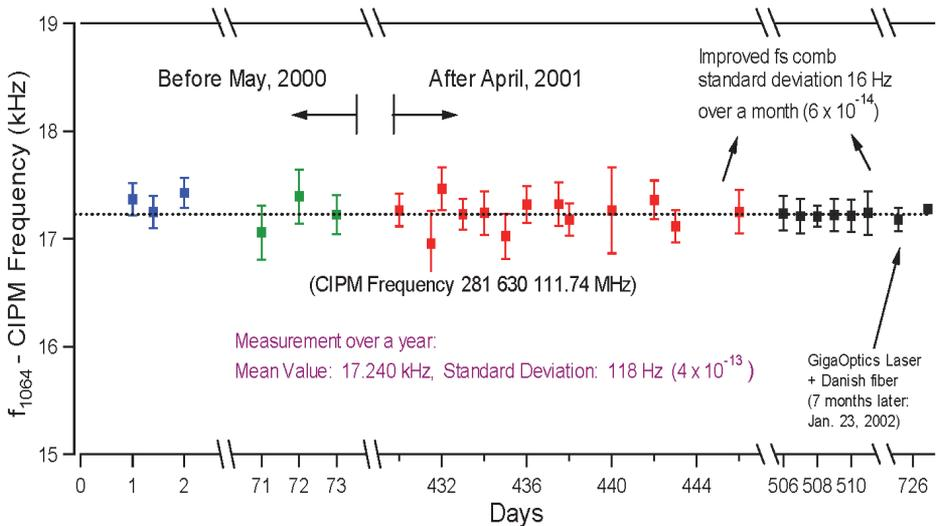
Fig 4. Long-term frequency stability of Iodine-based Optical Clock. This figure conveys the refinement and small frequency offset of this stable optical clock's frequency from previous, much less accurate measurements. With improved technology in 2002 the uncertainty was further reduced to  $\sim 6 \times 10^{-14}$ .
