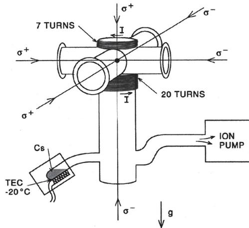
FIG. 3. The glass vapor cell and magnetic coils used in early JILA efforts to hybridize laser cooling and magnetic trapping (see Monroe *et al.*, 1990). The glass tubing is 2.5 cm in diameter. The Ioffe current bars have been omitted for clarity.
